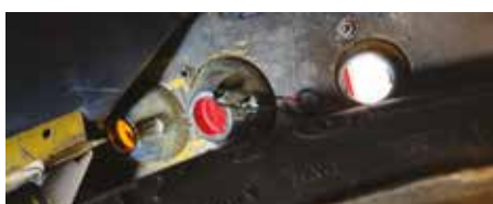
Light unit in place with the bulb holders removed, some of the fixing nuts are visible in the picture, there are five of them
