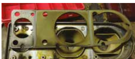
The foam rubber seal under the lenses
