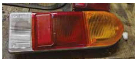
Lenses being replaced, the clear reverse lens in the picture is not fully slotted into the red stop/tail lens
