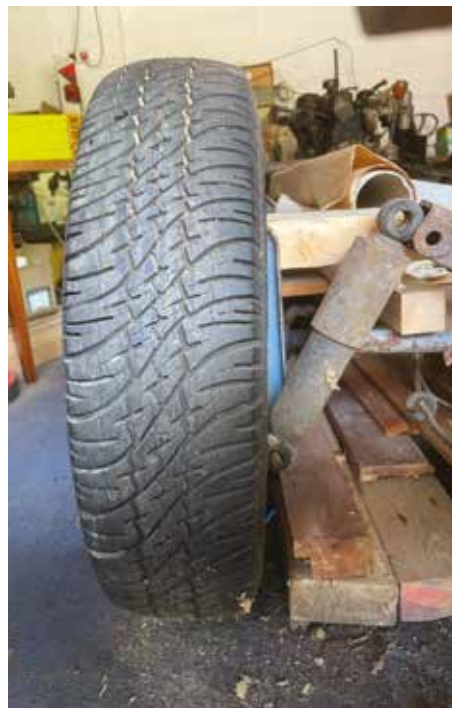
3 - Original damper at closed length showing limitation on suspension travel
