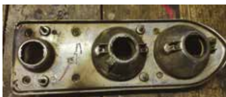
The light unit with the rubber seal removed exposing the six crosshead self-tapping screws which secure the lenses
